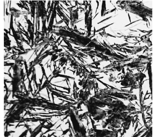
Typical martensitic microstructure (dark grains are BCT-martensite, lighter regions correspond to retained austenite ( \gamma )).
